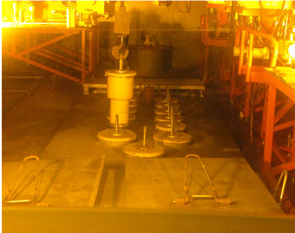
Figure B4: The Storage Pits at LEPI for Irradiated Experimental Fuel Rods and Fragments
